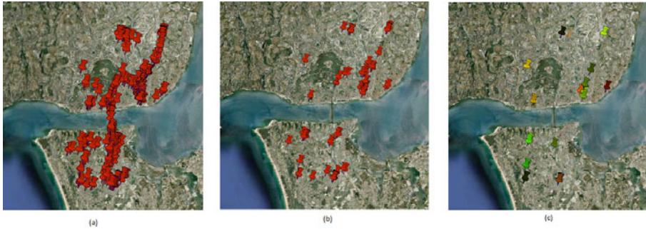
Fig. 1. Two weeks of a user location history: (a) all GPS points from the logs; (b) parsed stay points; (c) meaningful places
