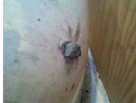
Fig. 4. A stone of the rail ballast hammered into a radome
