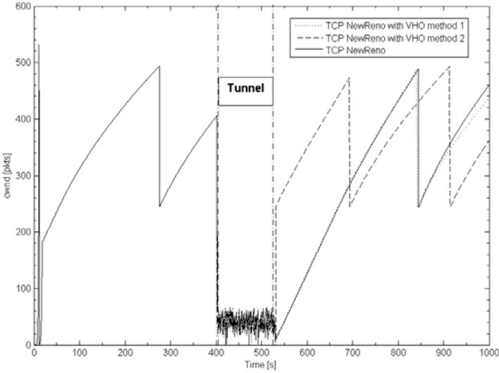
Fig. 7. Comparison of VHO techniques with TCP NewReno and single flow
