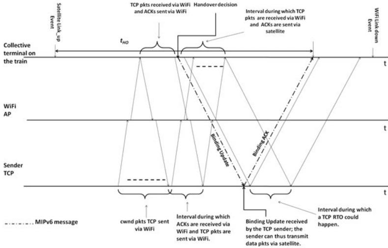
Fig. 3. WiFi-to-satellite VHO: scenario for maximum  $t_{HO}$
