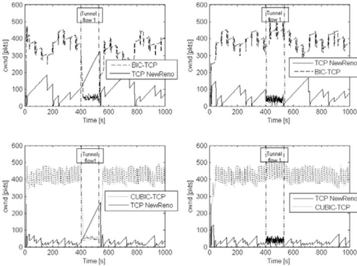
**Fig. 6.** Cwnd behaviors for two concurrent flows on two trains using different TCP versions (only flow #1 encounters a tunnel); no packet losses are considered
