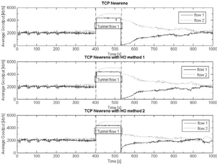
Fig. 8. Mean goodput for two TCP flows (only flow 1 encounters a tunnel)
