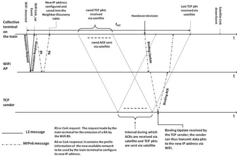
Fig. 2. Satellite-to-WiFi VHO: scenario for maximum  $t_{HO}$
