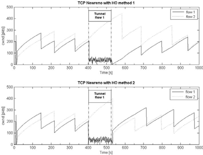
**Fig. 9.** Cwnd behavior of the two proposed handover methods used with TCP NewReno (only flow #1 encounters a tunnel); no packet errors are considered
