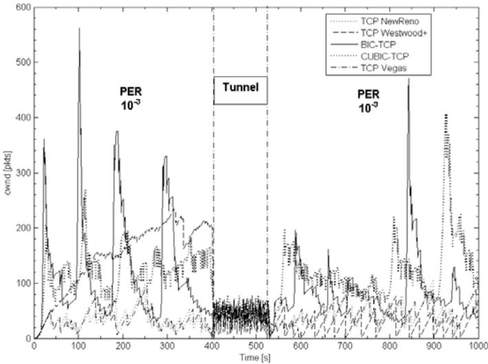
**Fig. 5.** Comparison of cwnd behaviors with different TCP versions in the presence of satellite-to-WiFi VHO (405 s) and WiFi-to-satellite VHO (525 s) VHO;  $PER = 10^{-3}$
