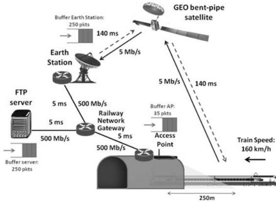
**Fig. 1.** Reference system architecture
