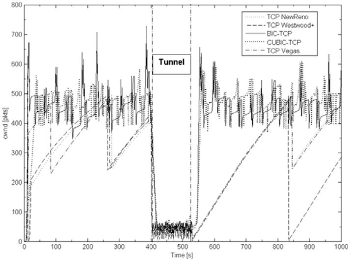
**Fig. 4.** Comparison of cwnd behaviors with different TCP versions in the presence of satellite-to-WiFi VHO (405 s) and WiFi-to-satellite VHO (525 s); no random errors
