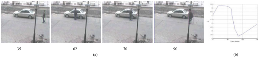
Fig. 4. Example of anomaly detection in the entrance/exit area of an office building. (a) An abnormal behavior where one people attempted to destroy the car parking the area. It resembles C3 in the early stage. (b) The behavior was detected as an anomaly from Frame 62 till the end based on Q_t .
