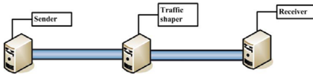
Fig. 2. Client-server based network used in the experiment
