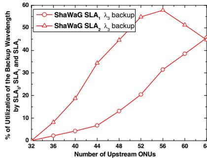
**Fig. 7.** Percentage of the wavelength utilization of the backup wavelength ( $\lambda_3$ ) versus the number of ONUs in ShaWaG to each profile
