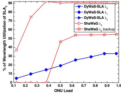
Fig. 5. Percentage of the wavelength utilization versus the ONU load for the SLA<sub>1</sub> for ShaWaG and DyWaS-SLA and 52 ONUs
