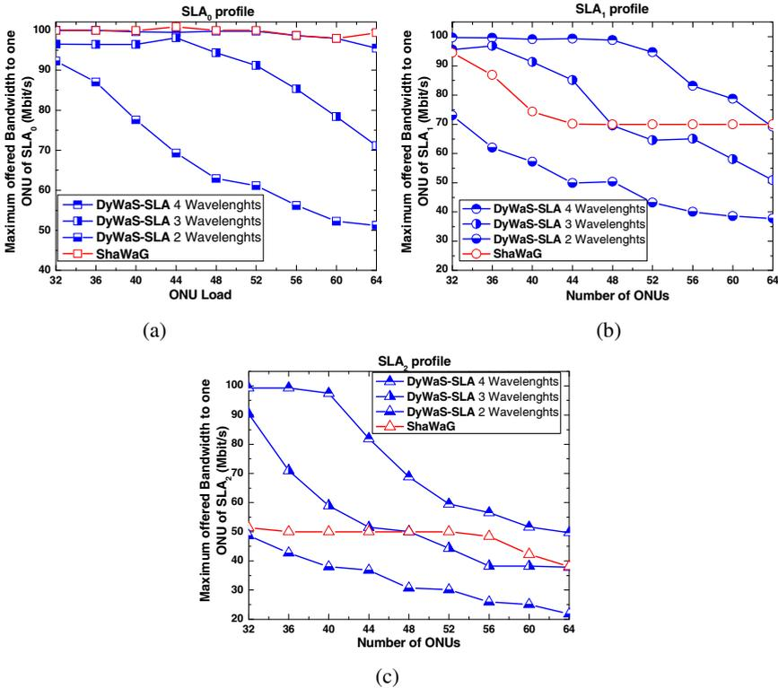
Fig. 8. Maximum offered bandwidth of DyWaS-SLA and ShaWaG to each ONU of each profile (a)  $SLA_0$  (b)  $SLA_1$  (c)  $SLA_2$
