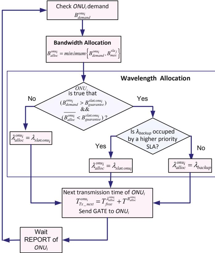
Fig. 2. Main diagram of the WDM-DBA algorithm
