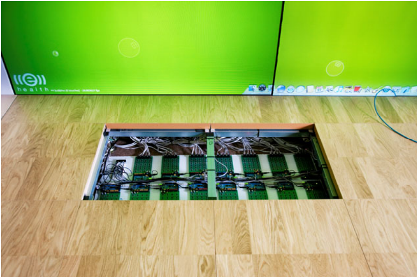
Fig. 2. Operation amplifier and microcontroller boards under the metal support structure for the sensors and the floor tiles
