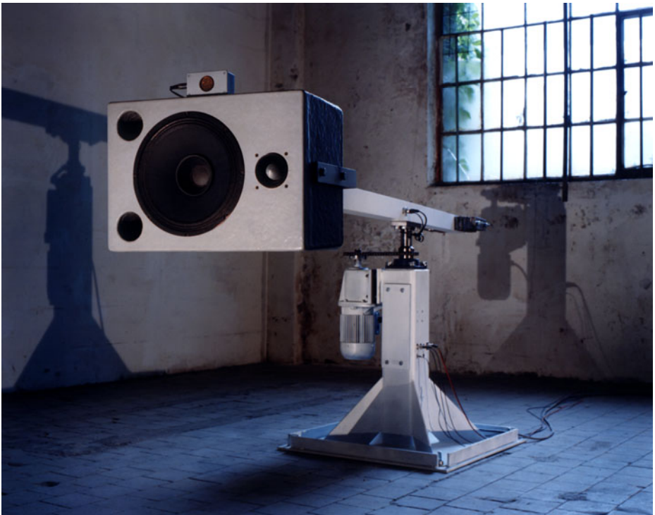
Fig. 1. The first prototype Spatial Sounds (100dB at 100km/h). This version is equipped with only one ultrasound distance measurement sensor.
