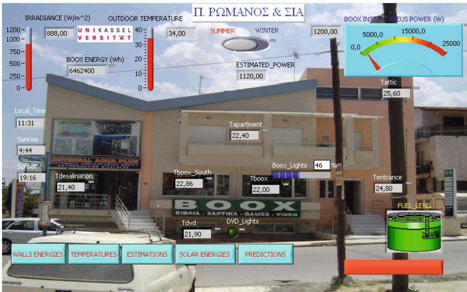
Fig. 3. The SCADA main window page
