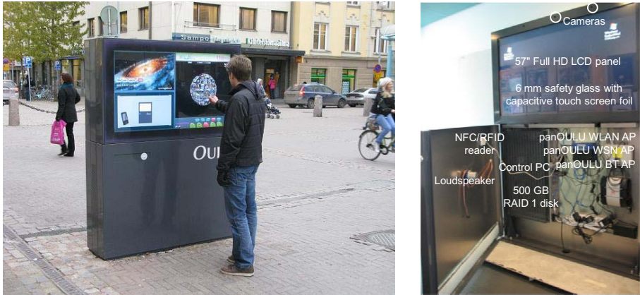
Fig. 3. (a) Outdoor UBI-display at downtown Oulu; (b) Components of an indoor UBI-display
