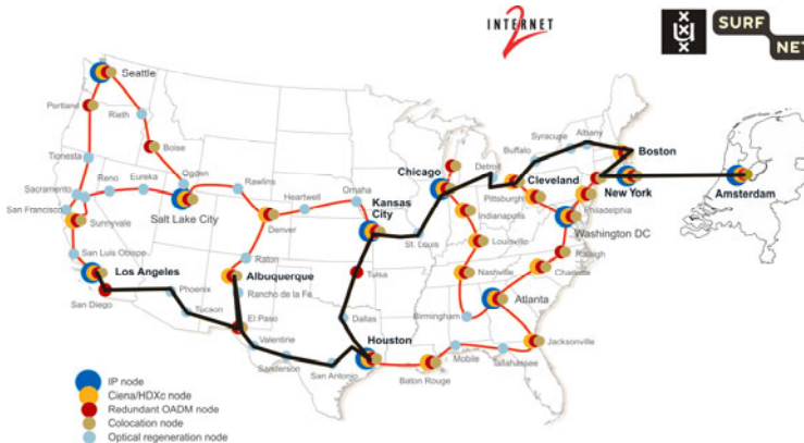
Fig. 7. The graphical overview of an end to end path realized with our software. In the specific case we created a dedicated circuit between Amsterdam and Los Angeles. This makes use of our service-plane to control-plane software.
