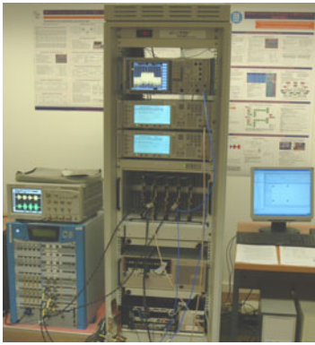
Fig. 8. CTTC real-time testbed. Left: channel emulator, oscilloscope. Rack: (top to bottom) spectrum analyzer, signal generators, RF frontends, baseband boards.
