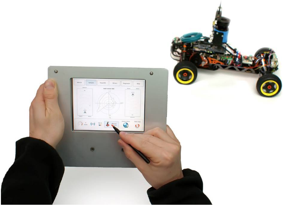
Fig. 2. Human-Machine Interface: Operation panel with color LCD display and touch screen. The controlled probe with sensors and actuator is in the back.
