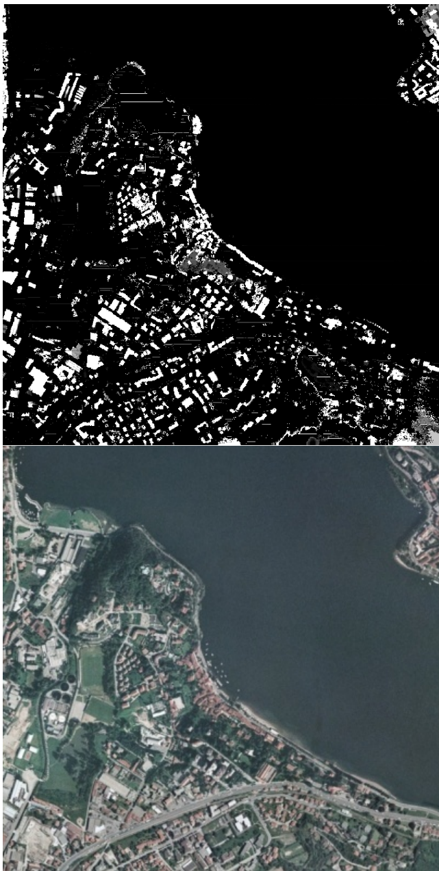
Fig. 5. Results of fuzzy buildings recognition (Above), the grey level are proportional to the output fuzzy value of the inference process. We can qualitatively compare the results to the aerial image (below) of the area.
