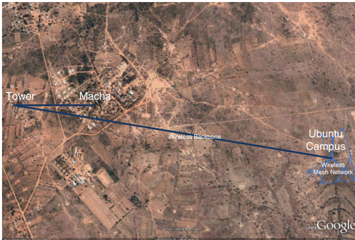
Fig. 5. Connecting Ubuntu Campus and distribute Internet access wireless
