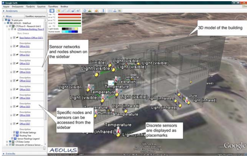
Fig. 3. Testbed at RACTI through Google Earth using Webdust
