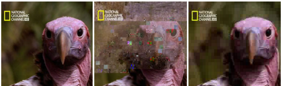
Fig. 6. By adaptation of IMS codec before Handover streaming can continue with reduced resolution (screen shot of video (a) before handover, (b) after handover without adaptation and (c) after handover with MRM/IMS codec adaptation)
