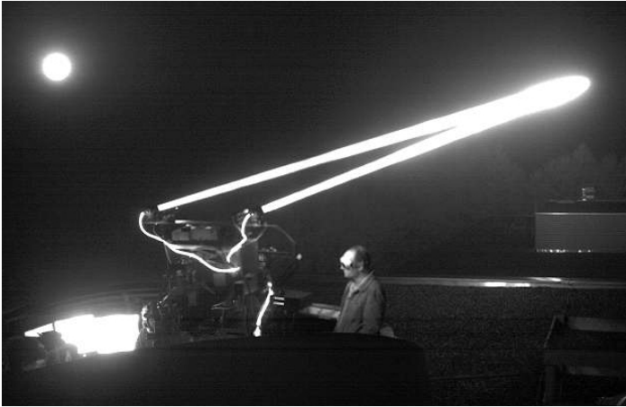
Fig. 11. Optical Ground Station Oberpfaffenhofen (OGS-OP) during the KIODO 2009 trials. Visible on the infrared picture is the beacon laser's backscatter due to haze.
