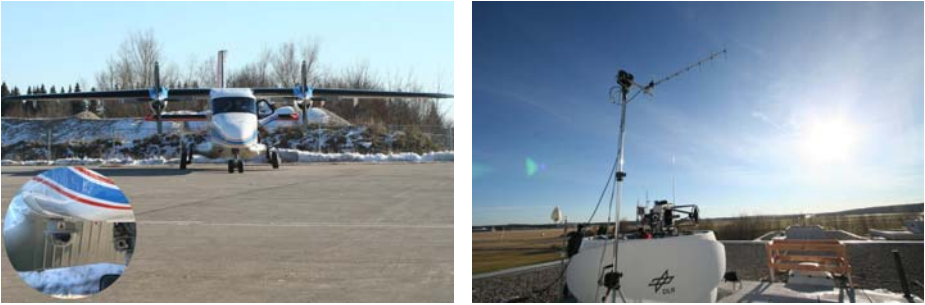
Fig. 5. Left: Picture of the Do228 Aircraft with installed Optical Terminal. Right: Picture of Optical Ground Station (OGS) with 40cm Cassegrain Telescope for data reception and an RF link antenna for reception of GPS data from the aircraft.
