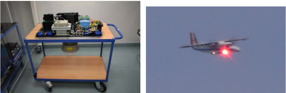
Fig. 6. Left: Optical Terminal in Lab. Right: View of Do228 aircraft during the trials. Visible is the red marker laser used for adjustment purposes.
