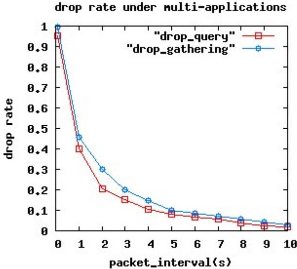
Fig. 4. The drop rate of two applications
