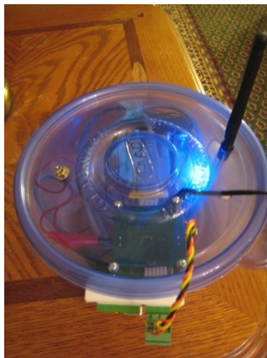
Fig. 2. Packaging of Oxybuoy electronics for the DO lab experiment
