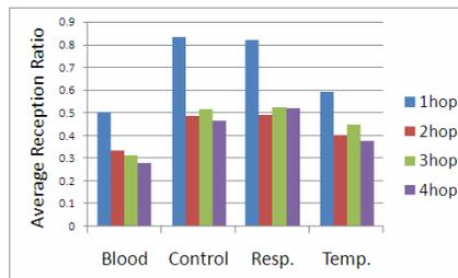
(b) average reception ratio for sensors of WBASNs positioned varying number of hops away
