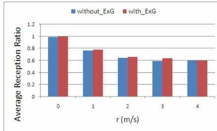
**Fig. 11.** Average Reception Ratio with varying travelling speeds
