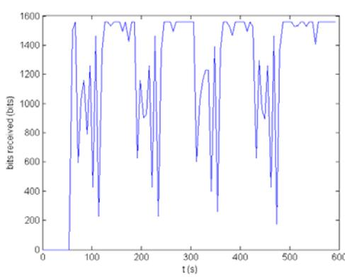
**Fig. 10.** An example of the bits received verses time when  $r = 1$  m/s and  $t = 60$  seconds
