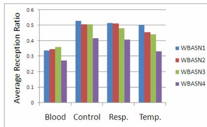
(a) average reception ratio for sensors of WBASNs positioned two hops away
