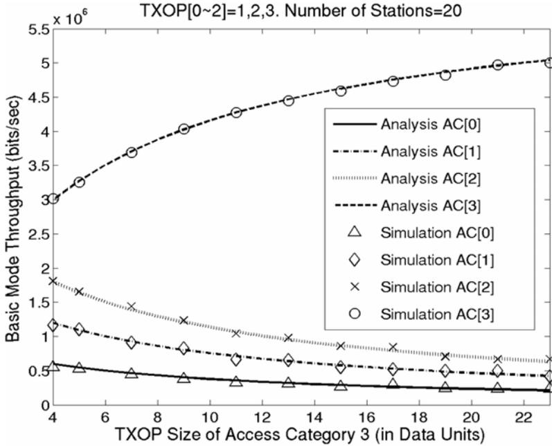
Fig. 6. Throughput of different ACs vs. TXOP[3] (basic mode, TXOP differentiation)
