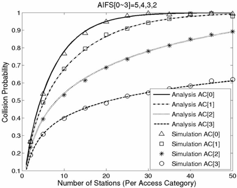
Fig. 5. Collision probabilities of different ACs vs. traffic load (basic mode, AIFS differentiation)
