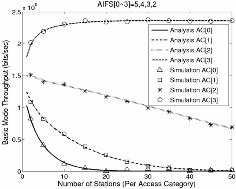
Fig. 4. Throughput of different ACs vs. traffic load (basic mode, AIFS differentiation)
