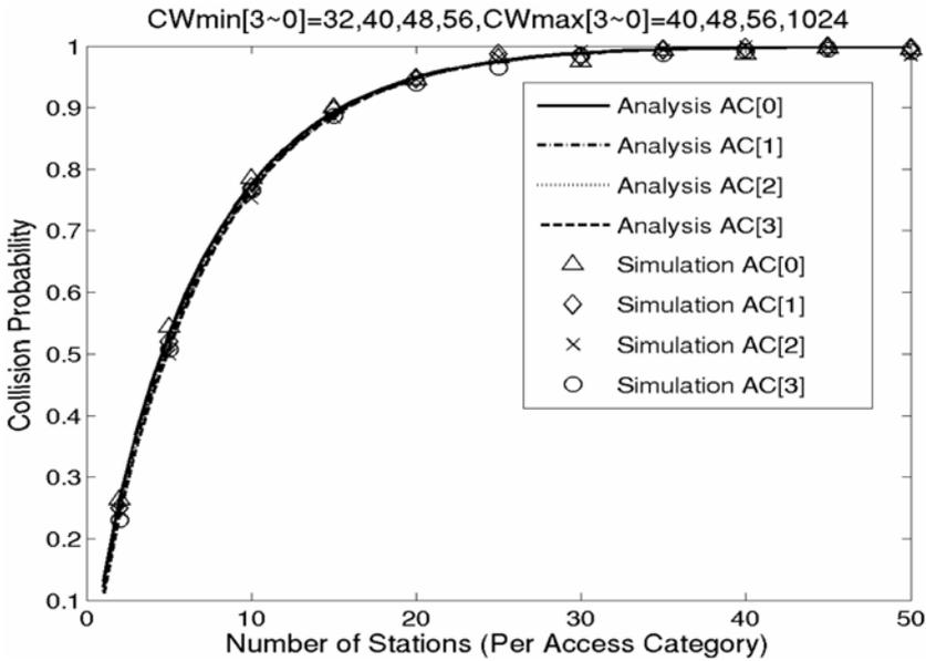
Fig. 3. Collision probabilities of different ACs vs. traffic load (basic mode, CW Differentiation)
