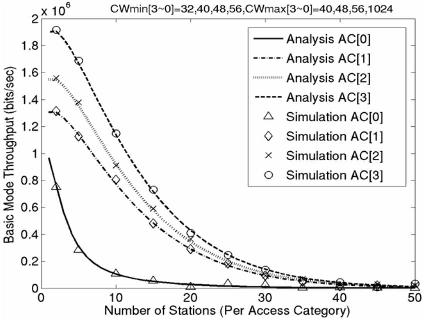
Fig. 2. Throughput of different ACs vs. traffic load (basic mode, CW Differentiation)
