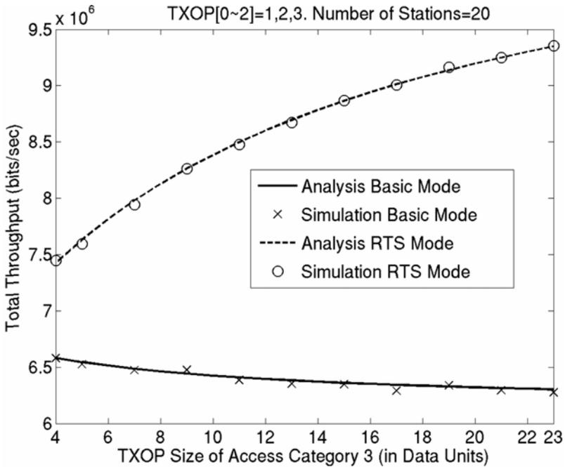
Fig. 7. Throughput of different ACs vs. TXOP[3] (RTS/CTS mode, TXOP differentiation)
