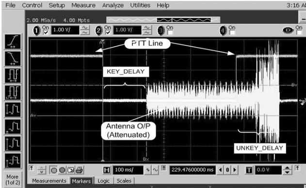
Fig. 2. Delay during keying (RTSI) and un-keying (TRSI) for a conventional analog radio
