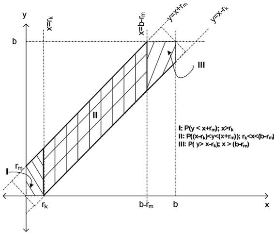
**Fig. 5.** Probability of collision between two nodes with different RTSI delays
