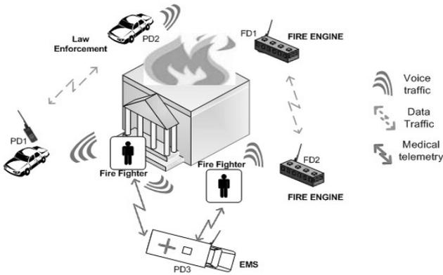
**Fig. 1.** Adhoc network based on digital LMR technology
