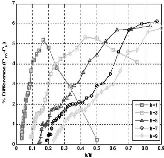
Fig. 8. Simulated Difference in the probability of collisions between m nodes and k nodes
