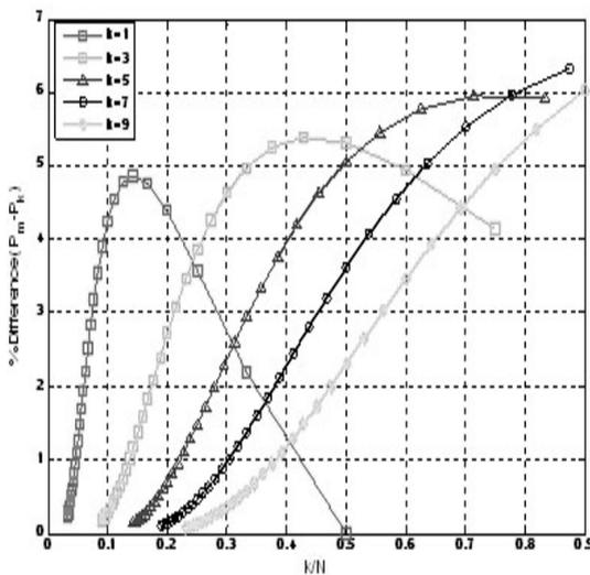
Fig. 7. Theoretical Difference in the probability of collisions between  $m$  nodes and  $k$  nodes
