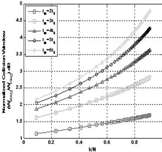
Fig. 6. Difference in the collision window sizes between  $m$  nodes and  $k$  nodes
