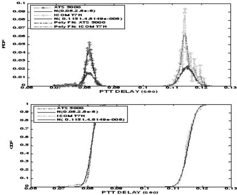
Fig. 3. Distribution of RTSI delays for Motorola XTS 5000 and ICOM IC-T7H
