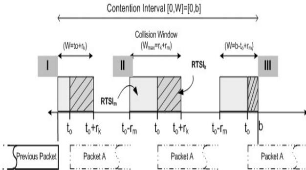
**Fig. 4.** Collision window for a single node
