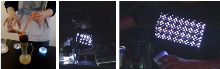
Fig. 5. The glass-layering interface (a) (50 x 240mm), costume display with graphic patterns (b, c), (260 x 180mm)
