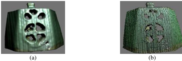
Fig. 6. (a) shows the surface recovered from densified correspondence. Comparing to (b) the reconstruction using original correspondence, the saw-toothed effect is quite unobvious.
