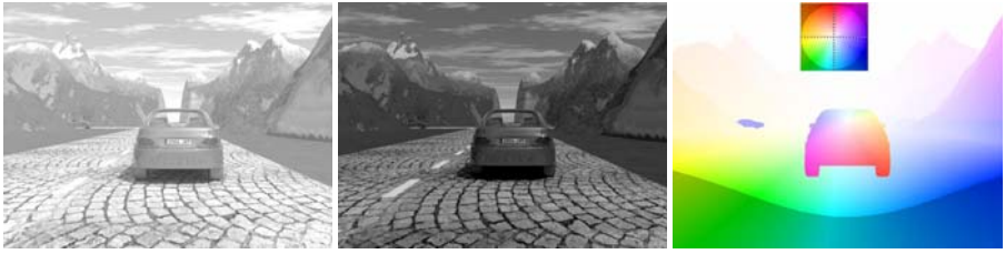
Fig. 1. Example frames from EISATS scene. Frame 1 (left) and 2 (middle) are shown with ground truth flow (right) also showing the color key (HSV circle for direction, saturation for vector length, max saturation at flow length 10).
