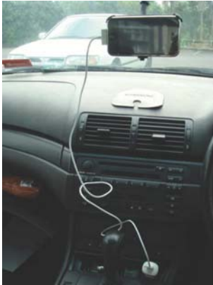
Fig. 1. Left: installation of iPhone on an ordinary car. Right: the geometry of road and camera.
