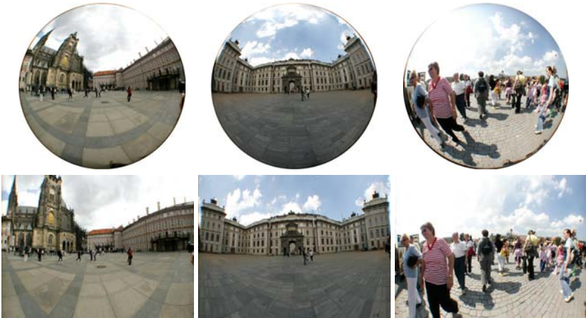
Fig. 2. Upper row: original fish-eye images (180-degree fields of view, showing Prague castle and a group of people). Lower row: resulting panoramic images.
