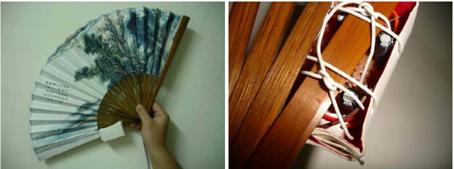
Fig. 9. A newer and smaller version of sensor is attached to the folding fan
