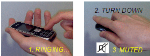
Fig. 1. Use case 1: TurnDown gesture use. Turn the phone display down to mute ringing.
