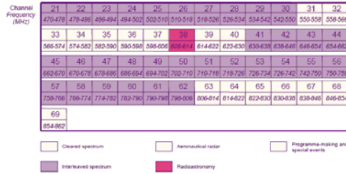
Fig. 1. The available VHF and UHF TV spectrum in the UK after digital switchover, showing both the interleaved (TVWS) and cleared channels [4]
