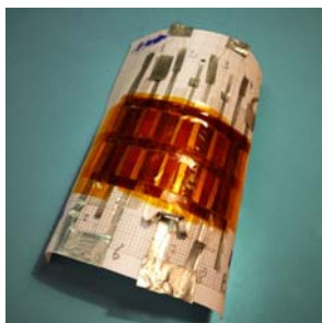
Fig. 3. Adaptive network with 8 organic memristors fabricated on flexible support
