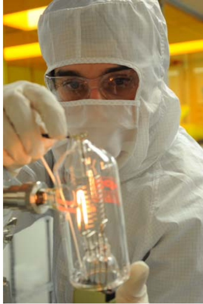
Fig. 1. Nanotechnology student working in class 100 clean room trouble shooting an ion gauge
