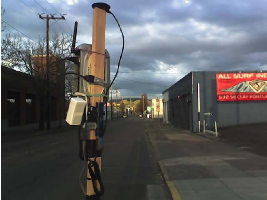
Fig. 4. Testing apparatus. A battery-powered Netgear WGT634u wireless router outfitted with a GPS device, USB storage, speakers, and an enable key.
