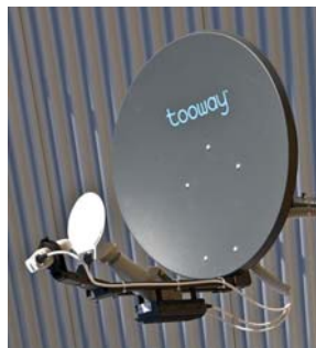
Fig. 6. Prototype of Ka & Ku bands Tooway™ ODU
