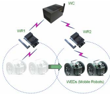
Fig. 3. Handover scenario for mobile robots
