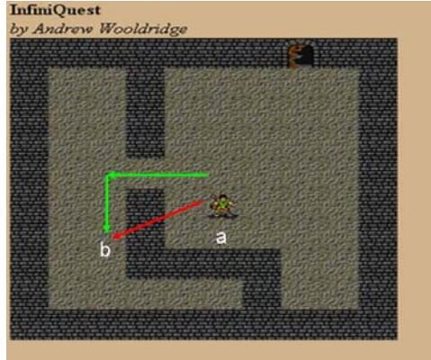
Fig. 1. Walking through walls: an example of semantic integrity violation. The central game server only keeps the coordinates of the two end points of a moving player as part of the abstract state, point a at (x_1, y_1) and point b at (x_2, y_2) . A cheating player may violate the game rules by walking through walls (the red path) without being detected by the state server.
