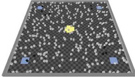
**Fig. 5.** Screenshot of the simulation scenario: Light-grey boxes indicate unloaded robots. Dark-black boxes indicate loaded robots. They move on a chessboard-like arena, where every grey square represents a patch. In the corners of the arena, four rectangular dirt areas (sources) are shown. In the center of the arena, a cross-shaped dump area (target) is shown. Robots should transport dirt particles from the sources to the target in as direct as possible trails.
