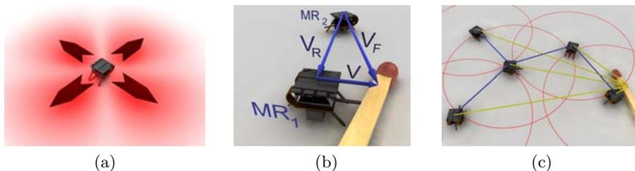
**Fig. 4.** (a) Representation of a theoretical emission pattern of the optical module mounted into the microrobot; (b) Vector sum for reconstruction of the direction of the target (e.g. a match):  $\mathbf{V}_F = \mathbf{V}_R + \mathbf{V}$ ; (c) Optical network established inside the swarm: darker vectors are the  $\mathbf{V}_R$  for each microrobot and define the forming trail; the circles defines the theoretical border of the communication range for each microrobot. © P. Corradi (2007)
