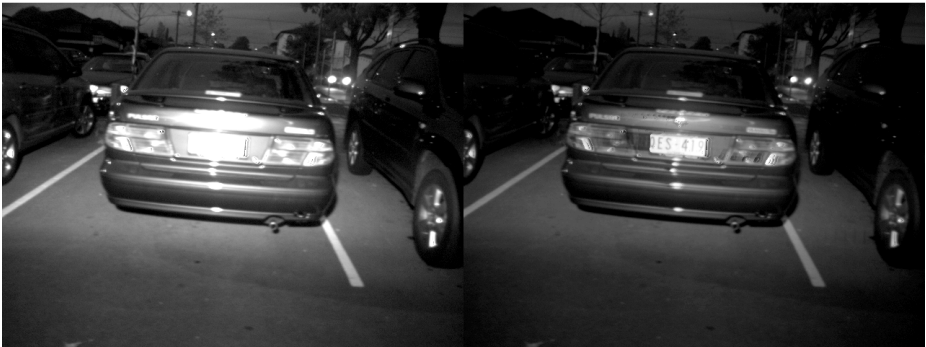
Fig. 6. Raw image (left) and improved detail after photoreceptor processing (right)
