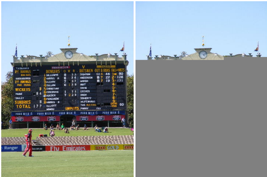
Fig. 2. The original image (left) was transferred from a laptop to an SD memory card. Although incomplete, it can be clearly seen that a significant proportion of the file was captured and reconstructed, resulting in a useable JPEG image fragment.
