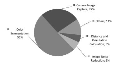
${\bf Fig.\,5.}\ {\bf Contribution\ to\ the\ overall\ execution\ time\ of\ each\ step\ associated\ to\ the\ Visual\ Landmark\ Recognition\ algorithm$
