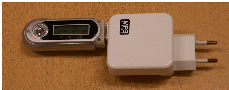
Fig. 2. MP3 player with an embedded FM transmitter, connected to power adapter. The antenna is not connected.
