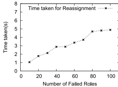
Fig. 6. Measurement of Time Taken to Reassign Roles in a Cluster Failure Scenario
