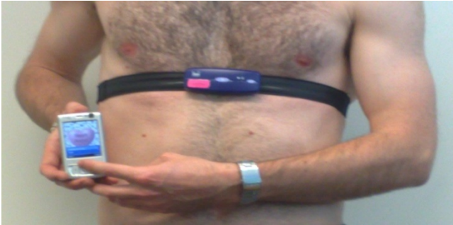
Fig. 1. Alive Technologies HRM Chest-Strap connected to phone via Bluetooth
