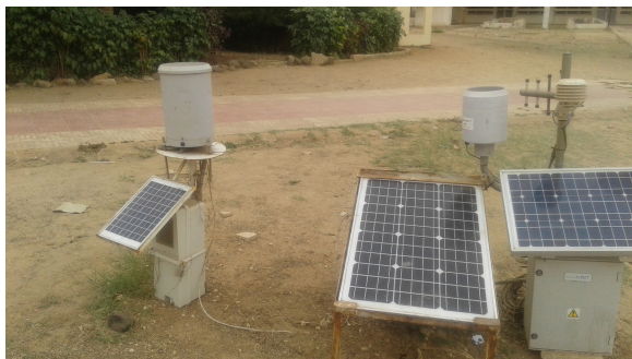
Fig. 7. Our automatic station designed (left) and Industrial rain gauge (right)
