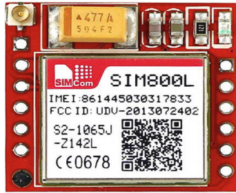
Fig. 1. The SIM800L quad-band network mini GPRS GSM breakout module used in the RWTMS.
