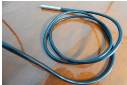
Fig. 2. The DS18B20 temperature sensor used in the RWTMS. (Source: Real-time, web-based temperature monitoring system for cold-chain management in Malawi)
