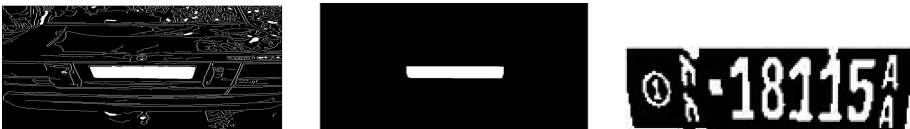
Fig. 5. LP detection and cropping. Image with LP candidates (left), Image with a true candidate (center), Image of a cropped LP (right)
