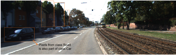
Box or rectangular selection of objects for labelling in a video frame.
