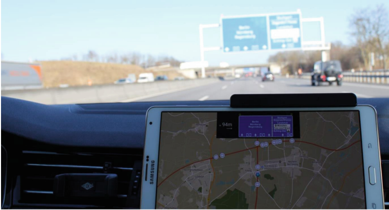
Fig. 3. Test application in vehicle displaying the same VMS as on the road (Source: Bavarian Road Administration).
