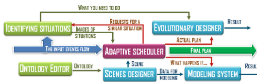
Fig. 2. The interaction between modules of the basic control system of the COTS
